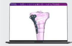
4. Design of the patientspecific plate along with the position and length of the screws.
